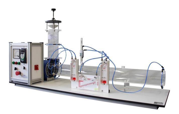
This equipment has been developed for the study of the characteristics of a centrifugal fan, through the realization of a wide range of experiments
